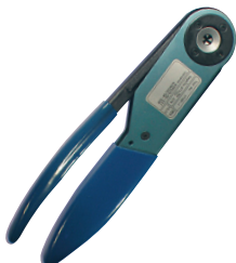
MANUAL CRIMPING PLIERS M22520/1-01
